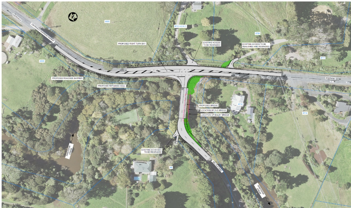
Figure 2: Proposed design for Two-lane Bridge and Right-turn Bay
