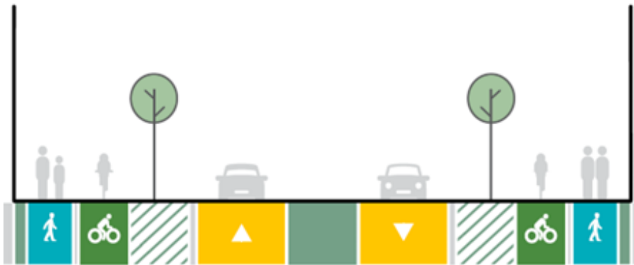
Figure 15-1 – Two-lane arterial as proposed for Popes Road and Croskery Road (indicative only).
