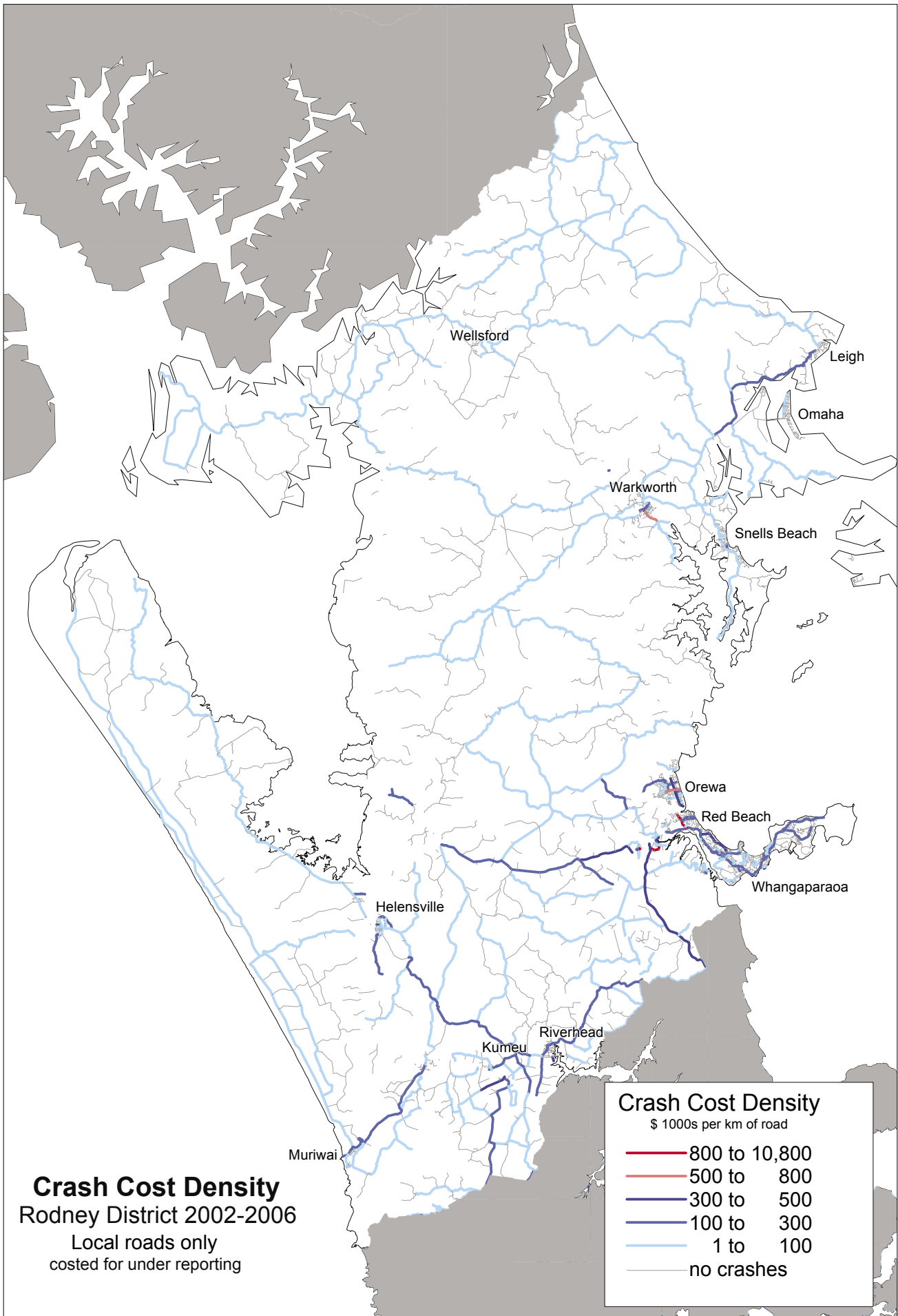
Figure 7. Crash cost density map for Rodney District, local roads only (Source: Ministry of Transport)
