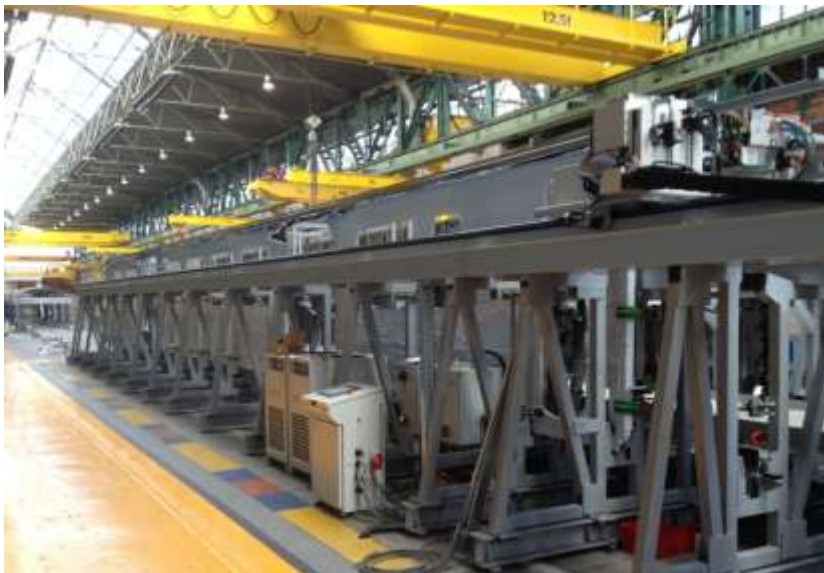
Figure 3: Bodyside panels in the jig, awaiting roof
