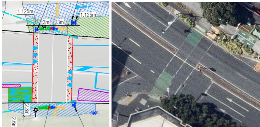
Figure 35: Mid-block Dual crossing connecting two-way directional cycleway and existing shared path (Source: Auckland Transport Project Drawing)
