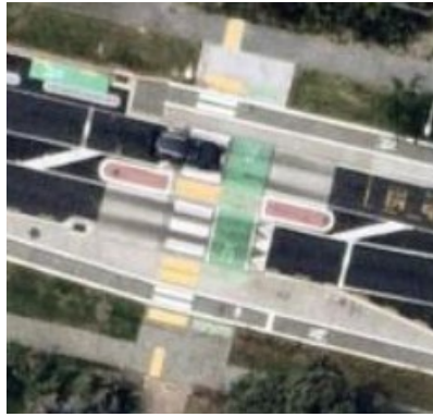
Figure 32: Mid-block paired zebra crossing, Taniwha St (Source: Auckland Transport)
