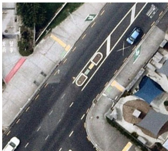
Figure 36: Refuge Island on pram crossing St Jude St, Avondale (Source: Auckland Transport)
