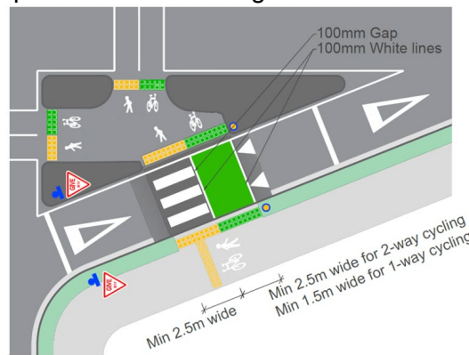
Figure 33: Paired Crossing – one-way traffic (Source: Auckland Transport)
