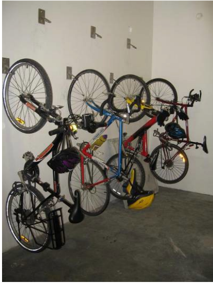
Figure 97: Wall hanging cycle racks (S Mills)
