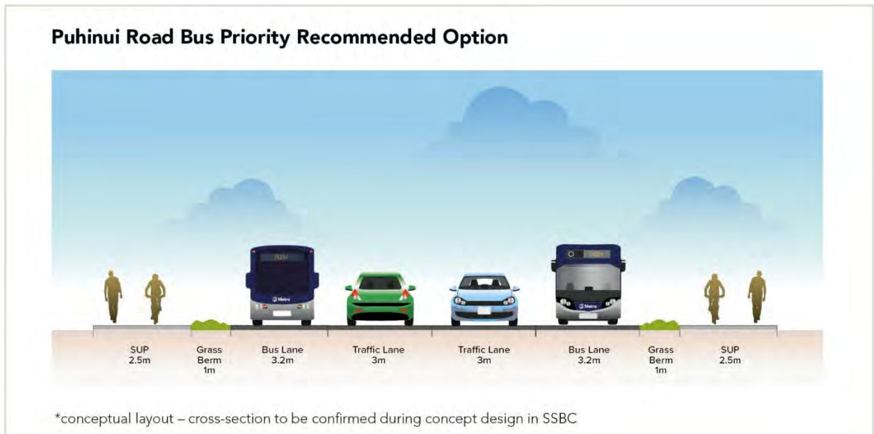
Figure 6-19: Puhinui Road Bus Priority Recommended Option cross-section
