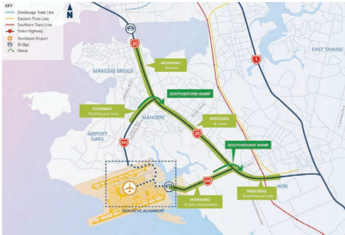
Figure 15-28: Recommended state highway elements
