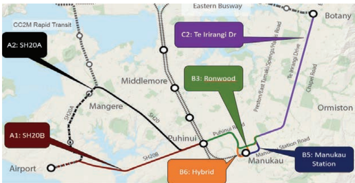
Figure 13-1: Rapid transit short list options summary alignments, including a ‘hybrid option’ in orange for the ‘B’ Segment.
