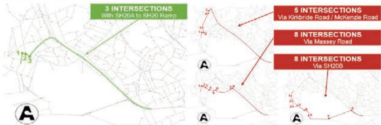
Figure 15-29: Intersections for a journey with (left) vs without (right) SH20A to SH20 ramp
