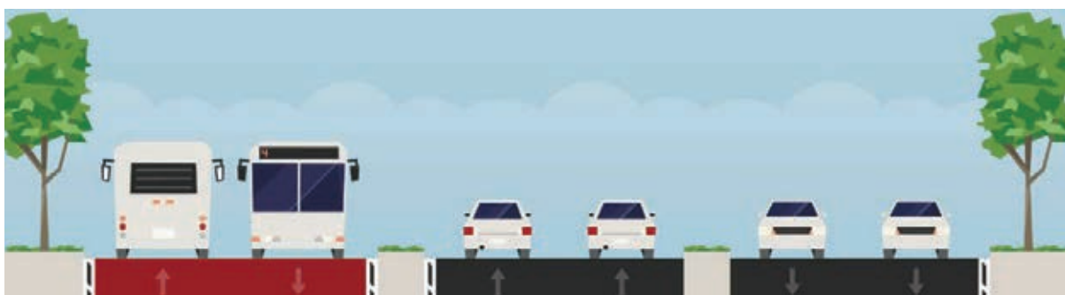
Figure 14-3: A-side running RTC route, the preferred placement for the Davies Avenue and SH20B section of the A2B corridor
