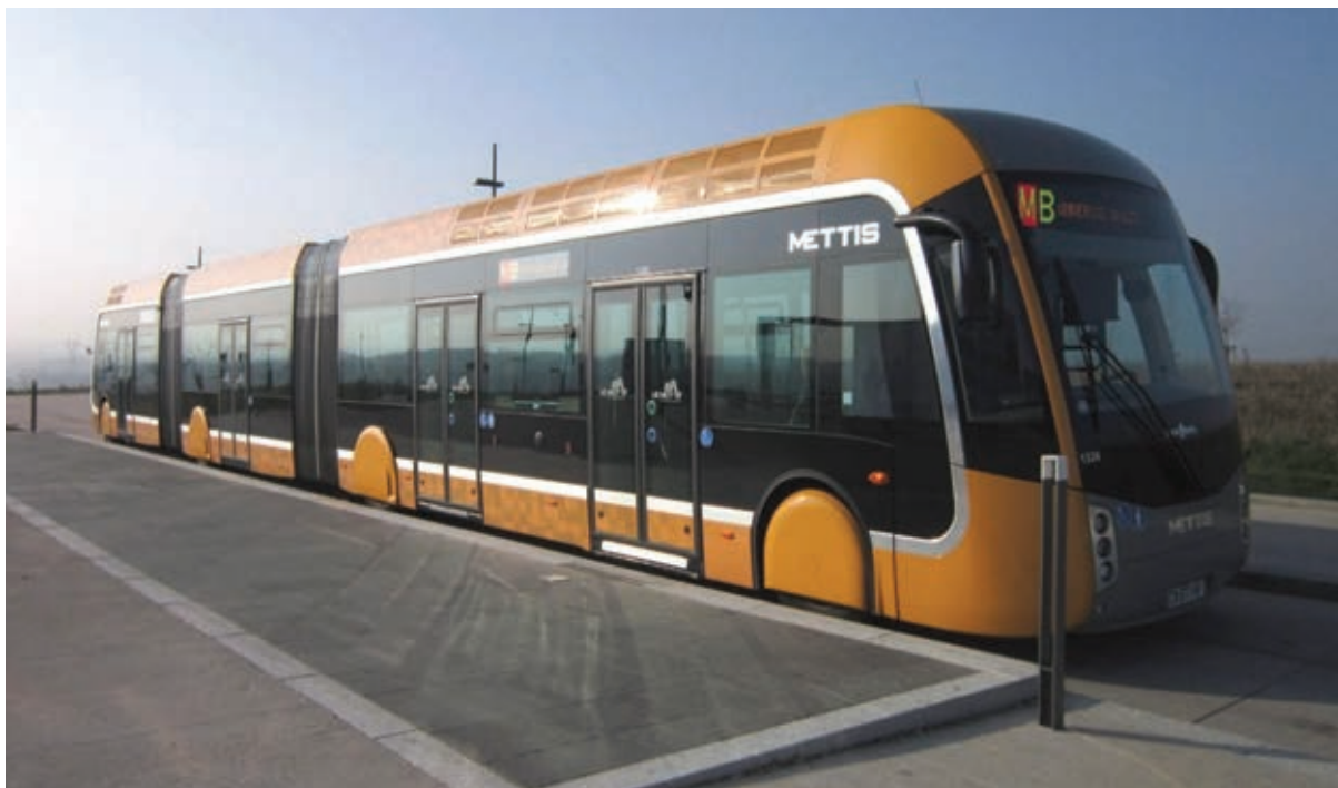
Figure 15-6: Example of high capacity BRT vehicle (double-articulated bus - Van Hool Exquicity) 24m
