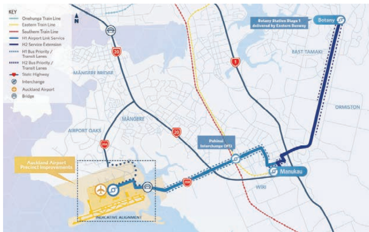
Figure 0-5: H1 and H2 service and infrastructure interventions
