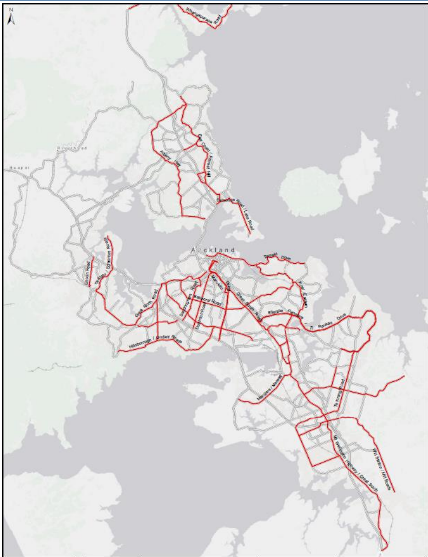
This map shows the 30 monitored arterial routes used to determine the average AM peak period lane productivity (2.4.1).
