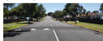
A speed hump is a short rounded raised section of the road. The white arrows indicate the raised surface and direction of incline.
