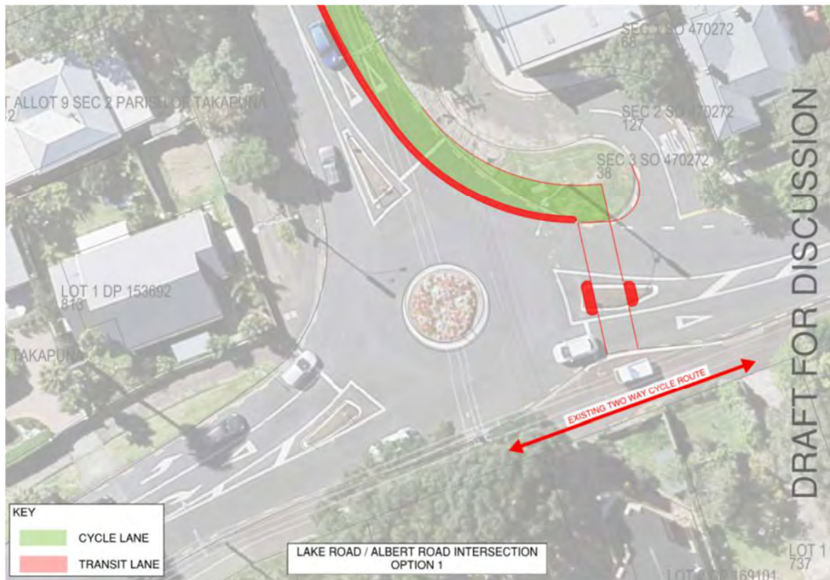
Figure 7-52 Lake Road / Albert Road Roundabout Option 1
