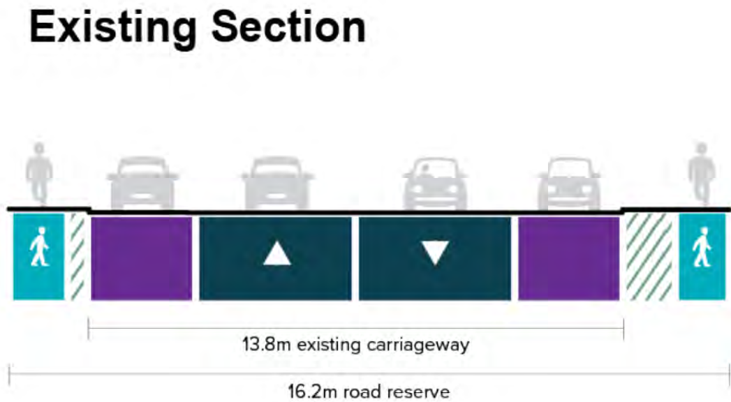
Figure 8-11: Western Segment – Existing Cross Section
