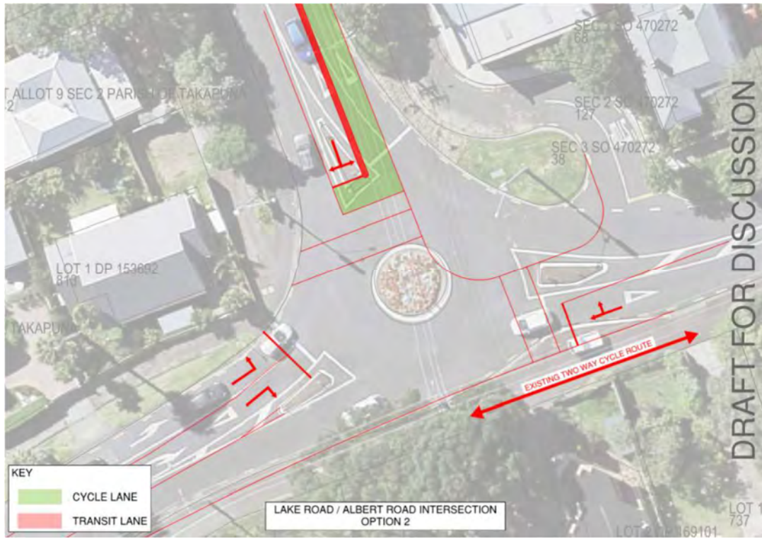
Figure 7-56 Lake Road / Albert Road Roundabout Option 2
