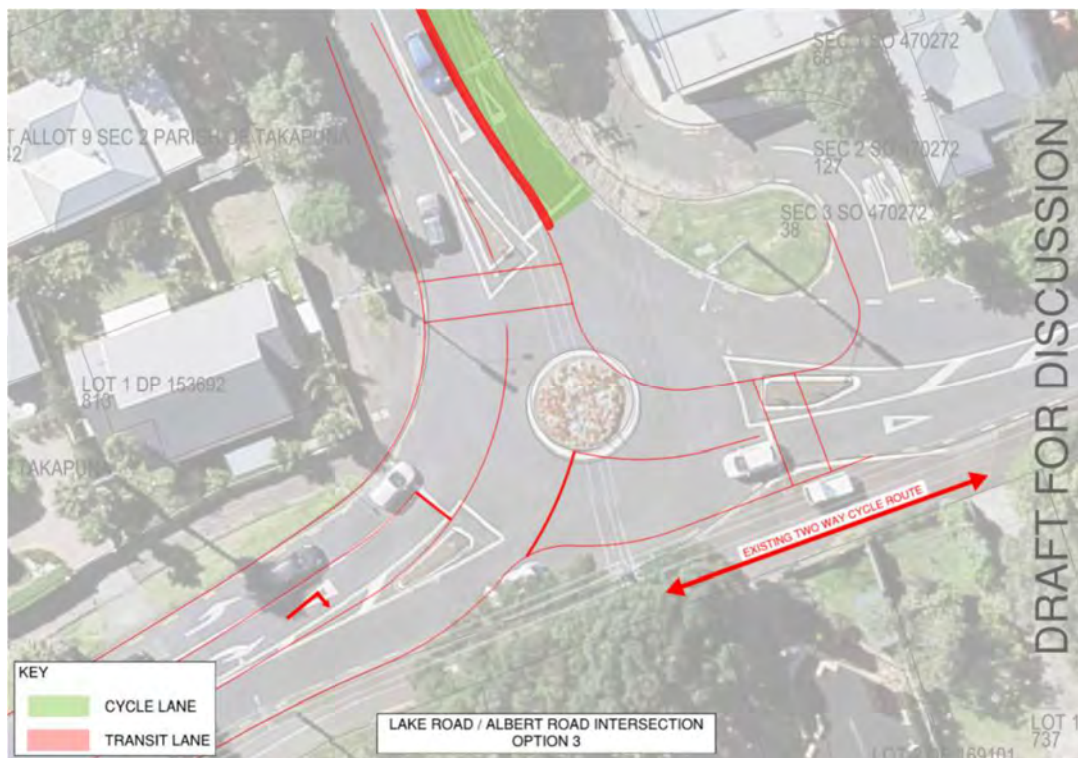
Figure 7-57 Lake Road / Albert Road Roundabout Option 3
