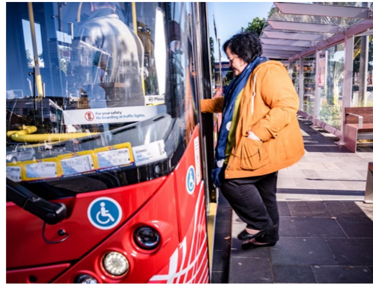
Small gap between the kerb and bus floor make it easy for passengers to board or alight.
