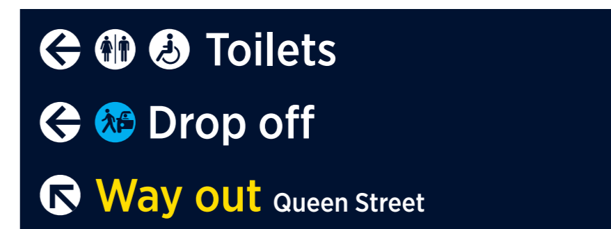
Fig. 1. Way out wording is positioned beside the arrow, is Yellow and always positioned at the bottom of the left or right block of directions.
