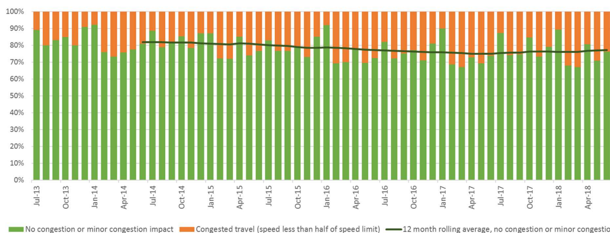
Figure 6-13: Proportion of morning peak travel on the arterial network by level of service (orange = congested)
