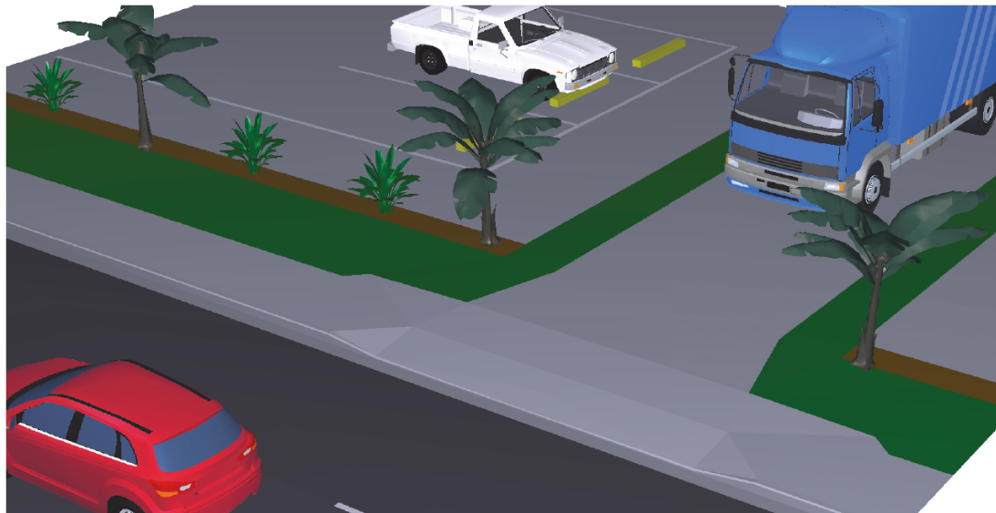
VEHICLE CROSSING WITH FOOTPATH <1.8m
