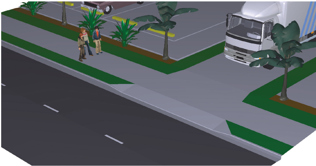
VEHICLE CROSSING FOOTPATH SEPARATED FROM KERB
