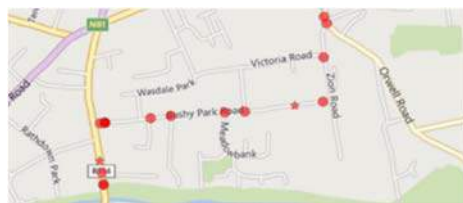
After intervention – more green time given to side road leading to more even headways
